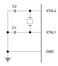
Notes: C1, C2 = 30 pF  $\pm$  10 pF for Crystals = 40 pF  $\pm$  10 pF for Ceramic Resonators
